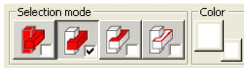
The four *Selection mode* buttons refer to selecting the *whole model*, *one shell*, *one surface*, or *one gap/triangle*, respectively. Now try to select a shell from the display area, such as the *1. slider (IGES Input)*. The *Selection mode* is on *Shell selection* by default but if not **press** the
