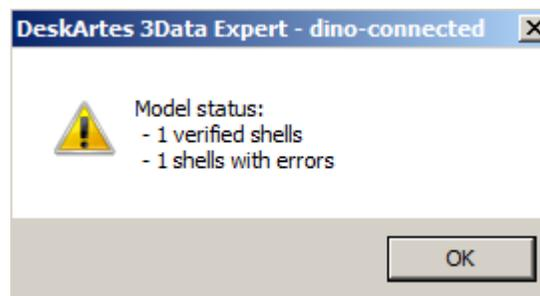
The message indicates that there is one verified shell, which also contains errors. The display shows red *Gap curves* through the surfaces. Gaps are an error type you must fix during the repair process.
