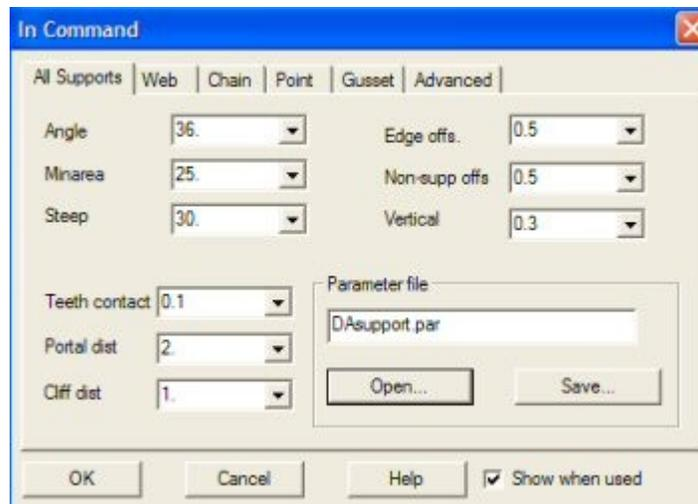
This set of parameters should get you started with the support generation. Anyhow, the exact values depend on the machine and the used resins. Testing, your own expertise and machine documentation will tell the correct values for each machine/material type.
