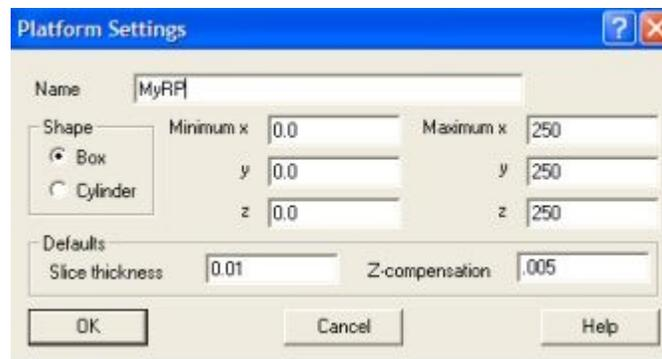
In this example we have selected the *size* to be 250x250x250 mm. The *slice thickness* is set to 0.01. This value depends on the specifications of your RP machine. The slice thickness here is used with the *Print Preparation > Slice* command automatically. The *Z-compensation* value is used with the *Print Preparation > Z-compensation* command automatically.
