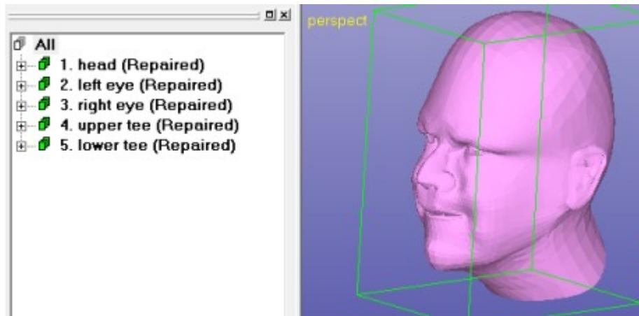
Now we are ready to combine the three remaining components, *head*, *upper teeth* and the *lower teeth* into one solid STL part. First we will use multiple selection to select all parts and then run the *Modify Faceted > Multiple Join* command on them.
