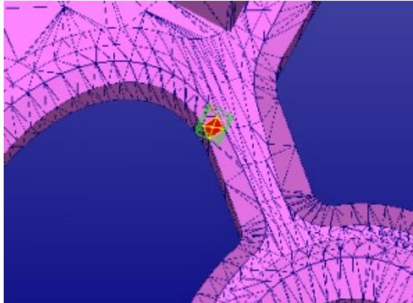
You will need to remove two small error surfaces in this area to get the result suitable for subsequent automatic repair shells command, i.e. model with small gaps:
