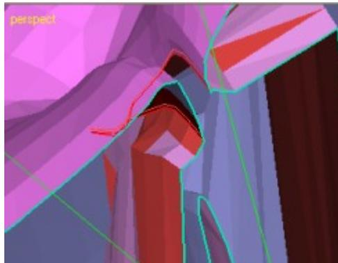
We can see that both the disjoint shells are more or less at the same distance from each other along the open edge. The approximate distance can be measured using the *Dimensions > Distance* command and it will give approximately 0.05 units (you can also use the
