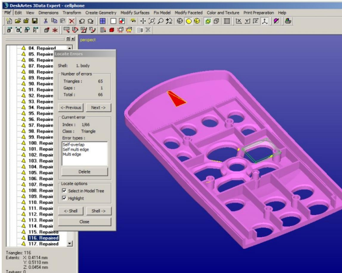
The Locate Errors dialog gives exact information on the currently highlighted error triangle (or gap), *Current error*. Also, the surface containing the error triangle is automatically selected in the Model Tree, as can be seen in the image above.
