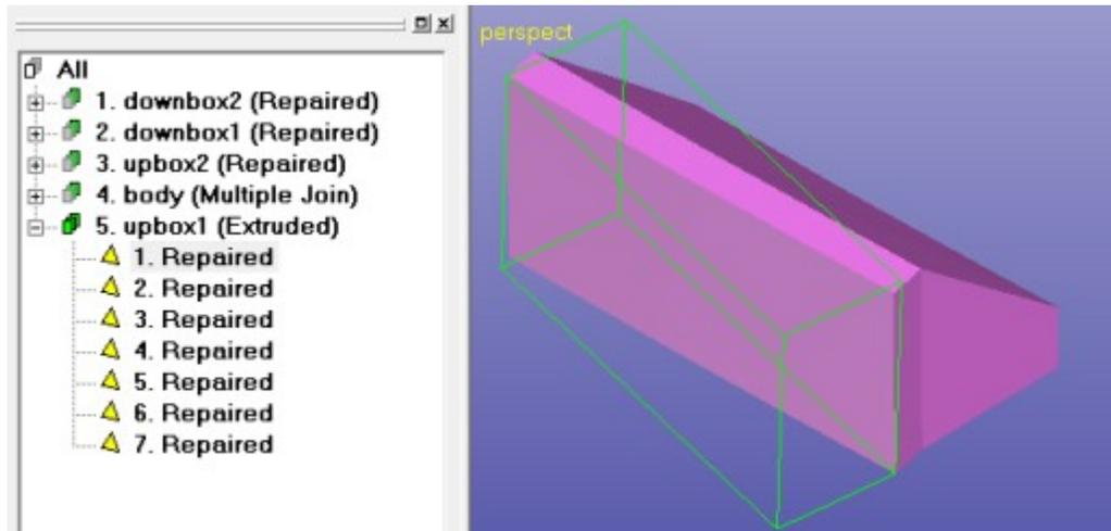
The command moves the selected surface to the (average) normal direction of the selected surface(s) and creates new edge triangles to keep the fixture solid. Now
