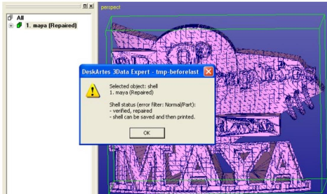
**Note:** You may find a new area or areas at the letter 'p' with similar errors after the last repair, just remove the *overlapping or intersecting* triangles in that case and rerun the Repair Shells once more. Or use *Fix Model > Edit Triangles* to clean up the error triangles, simplify the gaps and rerun the *Fix Model > Repair Shells* until there are no errors.
