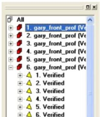
The Model Tree on the left hand side of the display area contains the directory to the geometrical information for the model. This model contains 6 *shells* (e.g. *1. gary\_front\_prof (Verified)*, ...). Each shell contains *Verified* triangle surfaces (press +-icon to see the *1. Verified*, *2. Verified*. etc. surfaces inside the first shell). The texture information for the VRML data (*.jpg* images) is stored after each surface.
