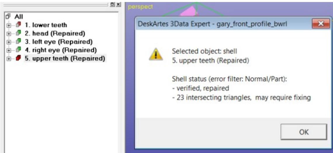
The software reports 23 *Intersecting triangles* error. A closer investigation (red triangles in the image below) shows that the intersecting triangles are are piercing through the outer surface.
