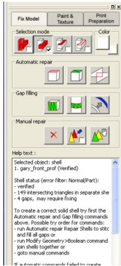
The input file is divided into 6 different shells in the Model Tree; the original head consist of these disconnected components (eyes, teeth, mouth ...). In the sequel, all gaps will be closed and the components will be connected into one correctly oriented part.
