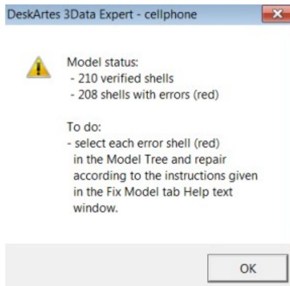
This indicates that most shells have errors and we should use Model Tree and Help Text to repair the model.
