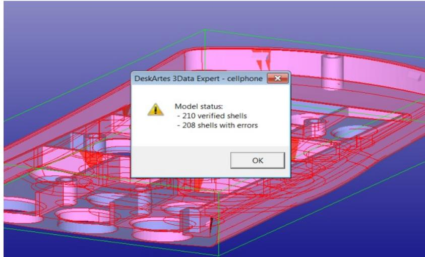
This is the result of the automatic analysis before the Auto Repair (the same result can be achieved through *Fix Model > Verify Shells* command if Operation Mode Window is not used).
