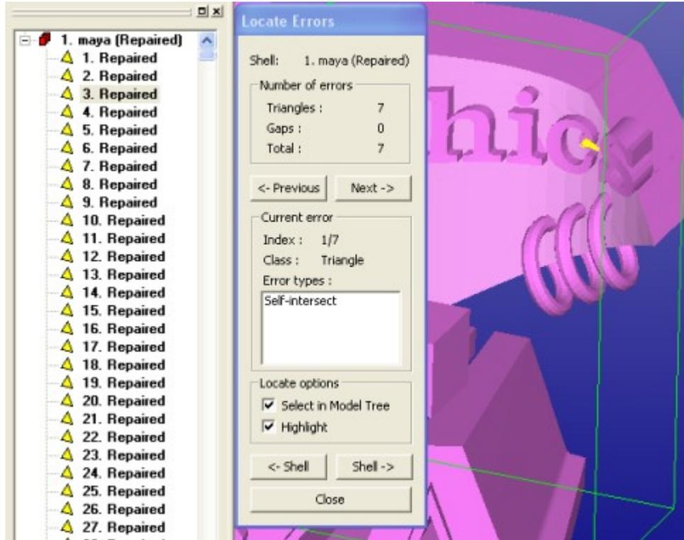
The last errors are at the letter 'c' in the graphics string. **Press Next** or Previous to zoom into the error area and the **close the Locate Errors dialog**. The errors around the letter 'c' are similar to the previous two errors we have fixed:
