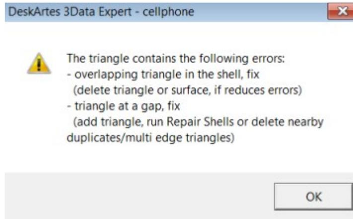
The dialog appearing will give more detailed information on the errors in the clicked triangle. We will follow the first help to remove triangles or surfaces to reduce errors.
