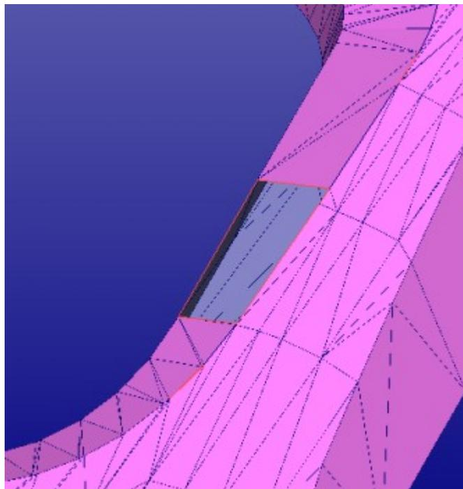
There is still one area with red triangles around. The body – cylinder intersection has created red triangles on top of the body part. If you use the right mouse
