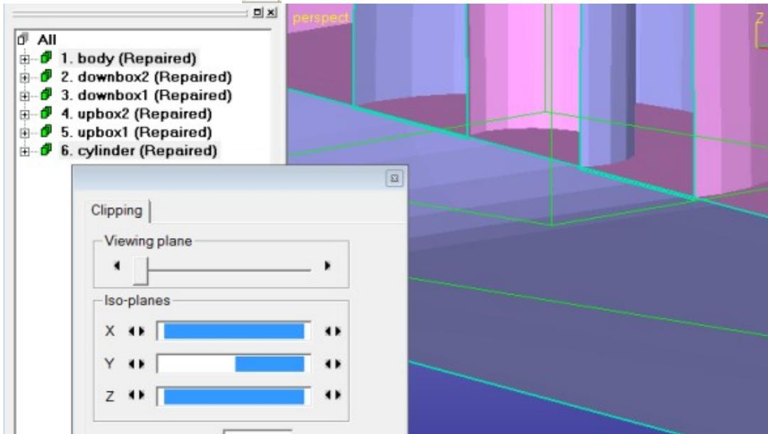
We can connect these two shells into one just by using *Modify Faceted > Multiple Join* or with *Modify Faceted > Boolean* command. We will use Multiple Join command.
