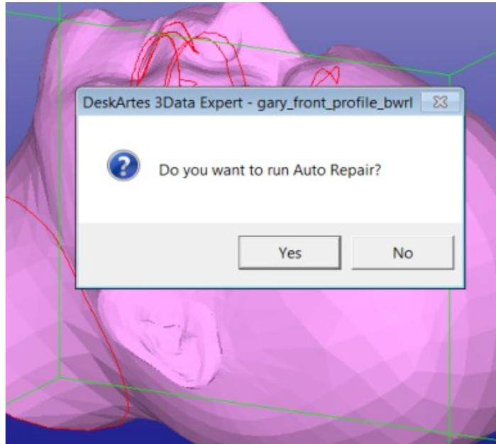
The visual inspection of the errors (gaps) in the model suggest that we should not run the Auto Repair. Auto Repair will repair each open shell (6) separately into a solid shell. The gaps in this model at the mouth / lip region show that closing them may generate separate shells where shells should be connected to each other at open edges (lips vs. mouth). Anyhow, you may do a faster repair just by running the Auto Repair now and skipping to the chapter *Repairing the teeth* on page 44.
