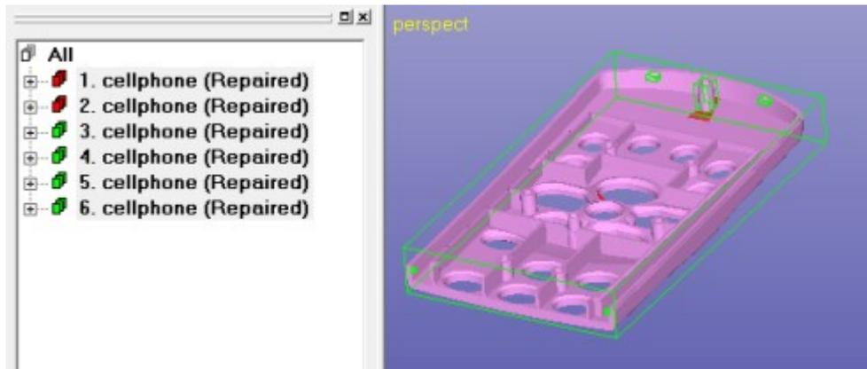
We have now managed to combine over 200 separate (open surface) components into 6 useful components. The next step is to repair each component separately to a correct STL file and then use the Boolean operations to form one final part. The next step is to first to repair each shell into green state and then use the Boolean commands to join them into one component.
