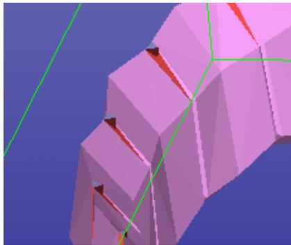
In the Fix Model Tab Help text window the most recommended repair action is to run *Remove Self-intersections* command.
