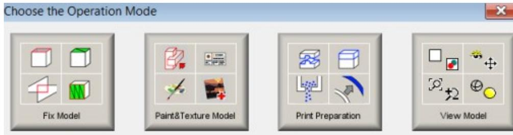
Operation Mode Window gives a reminder on the possible modification processes you can perform on a faceted model and allows you to select the correct set of tools for any operation. **Note:** if you do not see the Operation Mode window, please make sure the *Show operation mode dialog when opening a file* is *On* in the *Edit > Preferences General Tab*:
