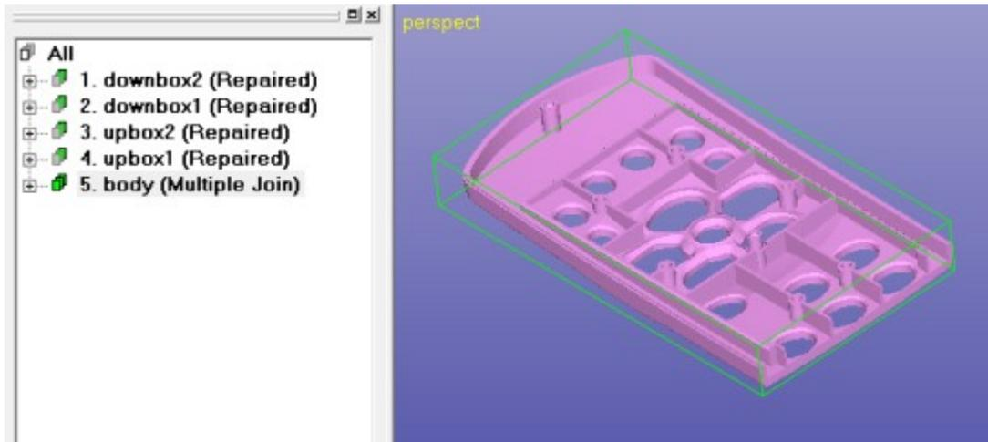
Now we will connect the *upbox1* and *upbox2* shells to the *body*. The fixtures are too far from the *body*, so we either need to move them towards the body or we need to generate extra material on the surfaces facing the body. Now we will generate more material on the surfaces. Extra material is added with *Create Geometry > Extrude Surface > from Surface* command.
