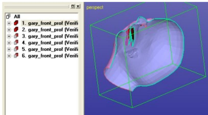
We can use different visual aids to define the order how to fix and combine the different components together (see the image above). Several viewing commands are available in the *View* menu as well as the Viewing Tab and Clipping Tab functions do determine the best way to go forward. For example, we can have a look at the model using clip form +X direction and a thick light blue clip curve, as seen above.
