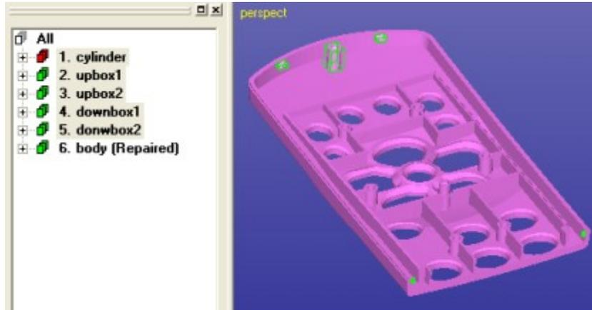
and run **Fix Model > Repair Shells** on all of them with the following parameters. Especially, the *Multiselected shells form separate parts* should be set *On* to keep the names for the results correct (and to avoid trying to stitch them together):
