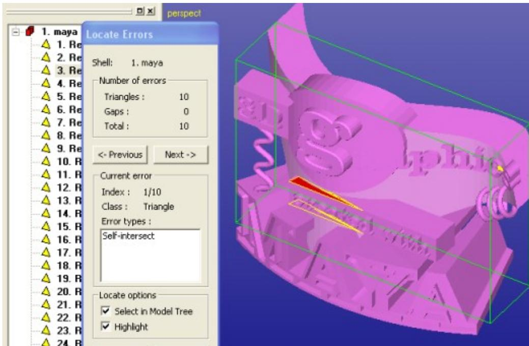
Press the **Next** button on the Locate Errors dialog until the following error triangle is highlighted on the screen:
