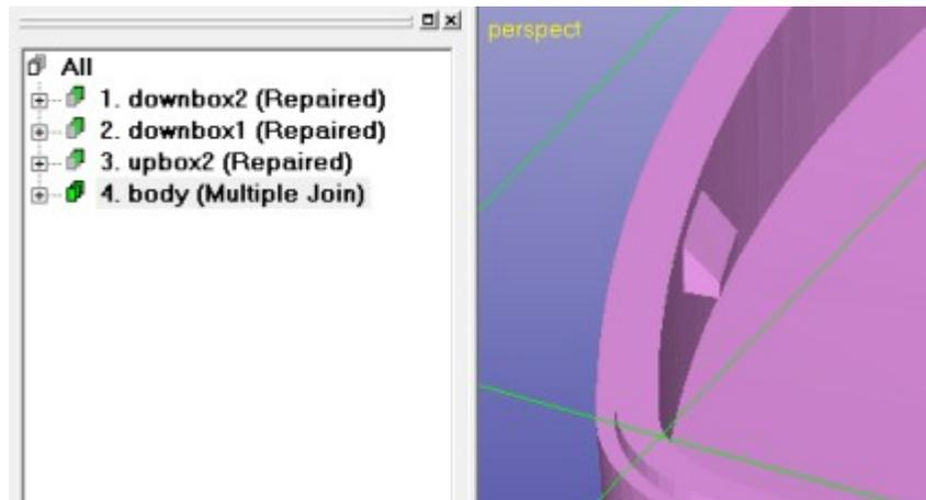
The result now has the two shells connected into one shell 4. *body* (Multiple Join). Connect the *upbox2* shell to the *body* in similar fashion,
