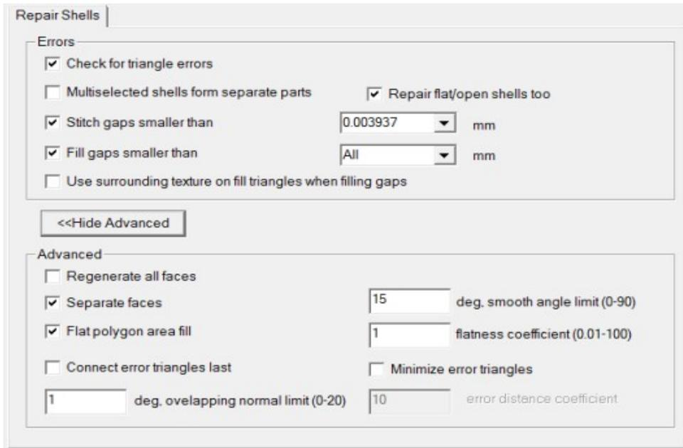
Flat open shells may be sometimes better to fix using Offset (or Join Gaps) to generate solid shells. Normal Auto Repair process does not try to fix flat open shell for that reason. But now we want to fix all shells we have selected i.e. stitch them to neighboring shells, so you make sure “*Repair flat/open shells too*” is ticked and
