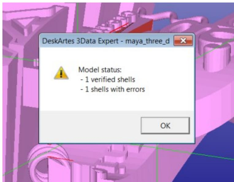
The normals are now consistently oriented and also the repair color is set to the normal sides of the triangles (the original material colors are stored for the 3D
