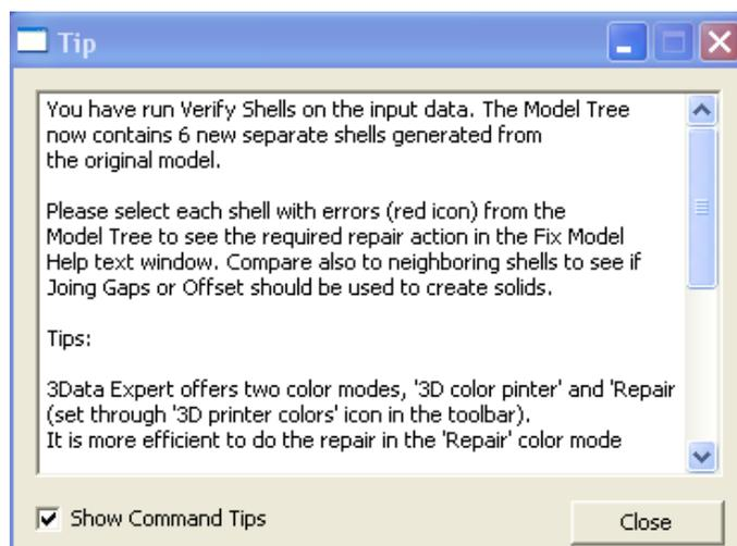
The Tip window gives useful information after different commands. For example, this tip window proposes to use the Fix Model Help Text window as well as visual checking to decide the next repair actions.
