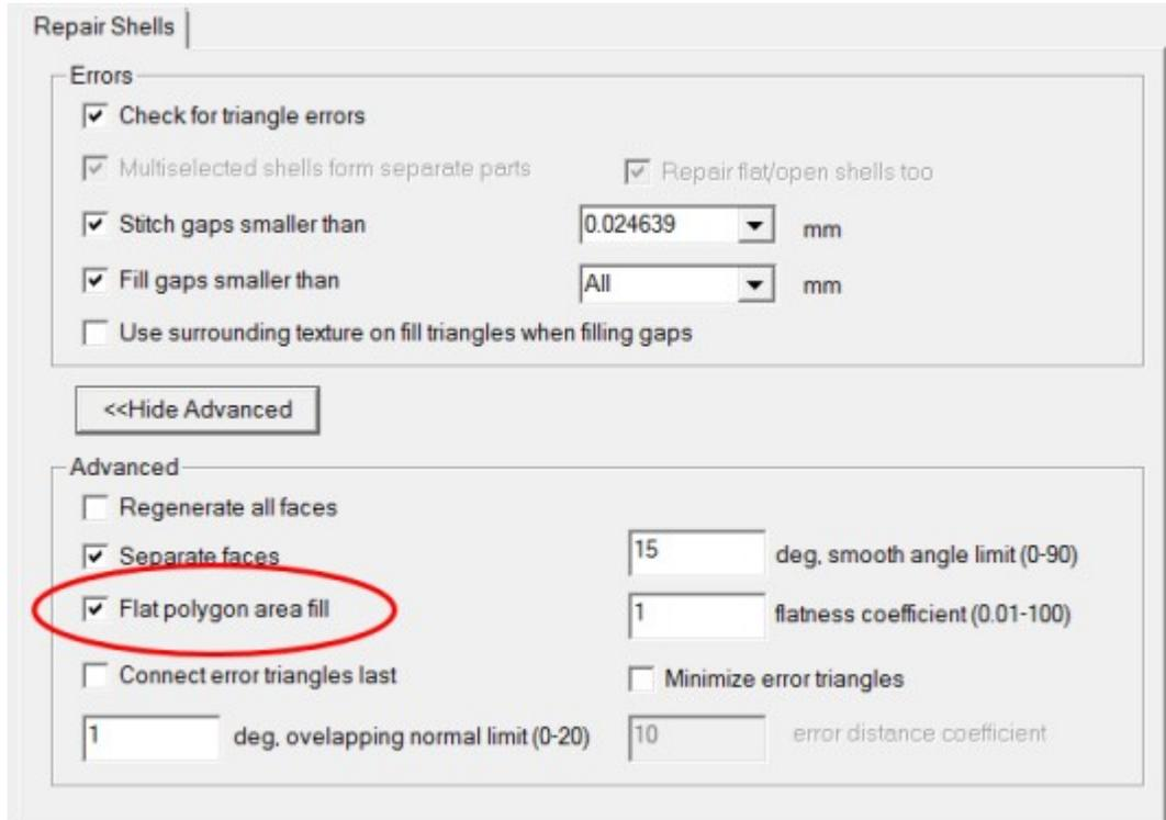
The new Flat polygon area fill, set on by default, will connect the flat gap polygons at the letter bottom edges to the surrounding box edges. All polygons lay in the same plane and the software use a special algorithm to fill between the separate polygons automatically.
