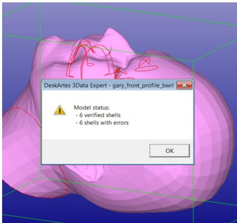
After the analysis the surface normals are corrected and the outer surface color is changed to pink, the inner surface color remains light blue.
