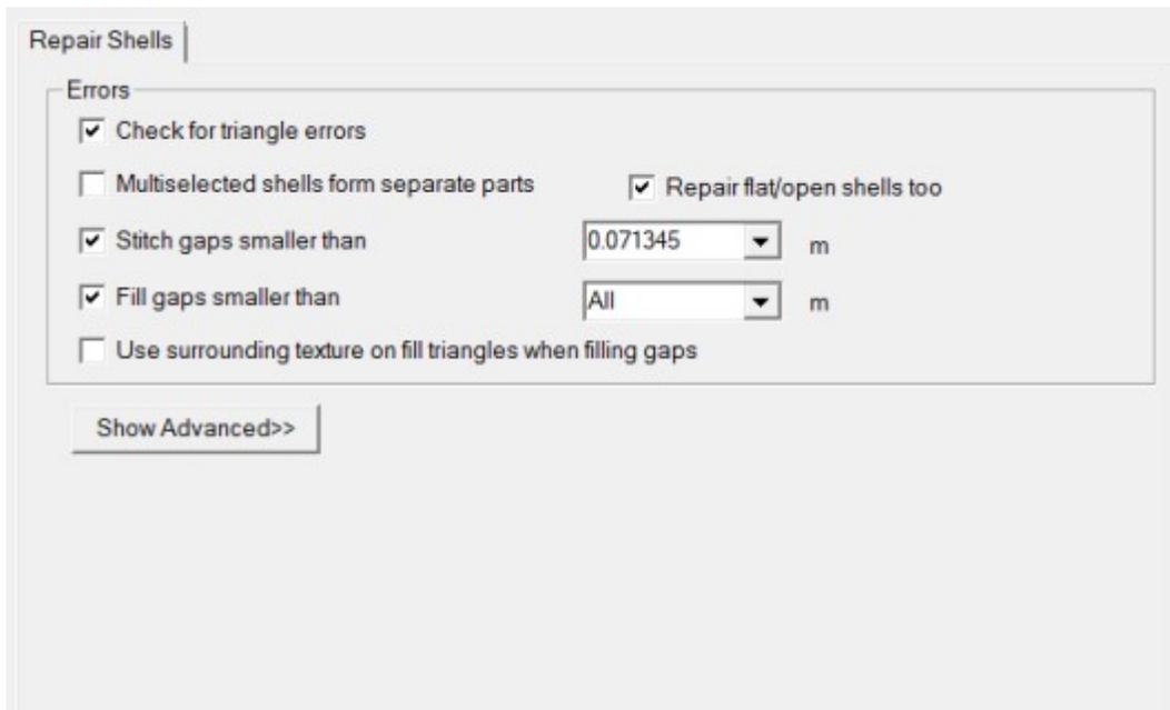
To get good results, we must give correct parameter values for the repair process. As seen above, normally we want *Check for triangle errors* as we are changing the geometry and we want to know the possible errors after the repair.
