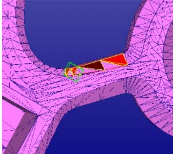
Select and remove surfaces until you have removed all bad surfaces in the area. You may also generate a larger gap at the area but do not worry, this will be filled with subsequent *Repair Shells* command:
