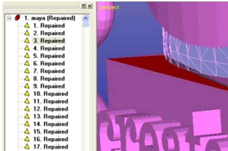
These errors can not be removed 100% reliably using automatic Remove Self-intersections command due to the tangential intersection conditions. Now we will remove a few triangles manually and then let the *Fix Model > Repair Shell* command to *Fill all* created gaps.
