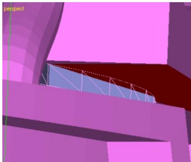
You may use the *mouse wheel zoom* and *middle mouse rotation* during the Edit Triangles command to get a better view to the delete triangles if necessary. After the removal the gap should look as seen here:
