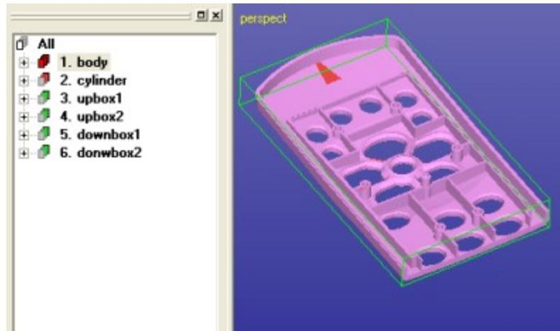
The *body* component has several errors due to the bad quality of the input data.
