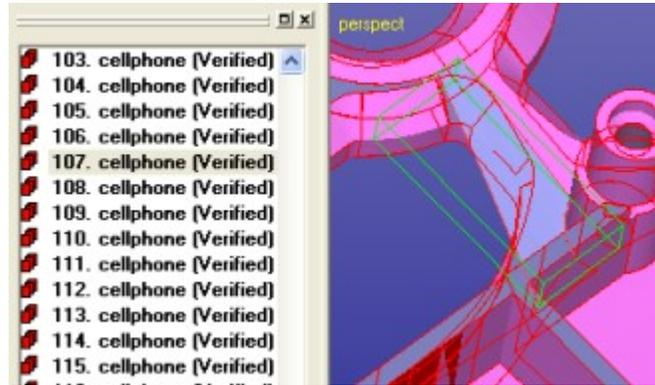
You may find more surfaces with errors (red areas indicating overlapping, intersecting, duplicate etc. triangles). You may sometimes remove more small shells or surfaces if you think are not needed when creating the correct model. Generally, very thin or flat surfaces can be removed, they will be fixed with gap stitching and gap filling later. Anyhow, with this exercise we will remove remaining errors using the help of *Fix Model > Locate Errors* command later.
