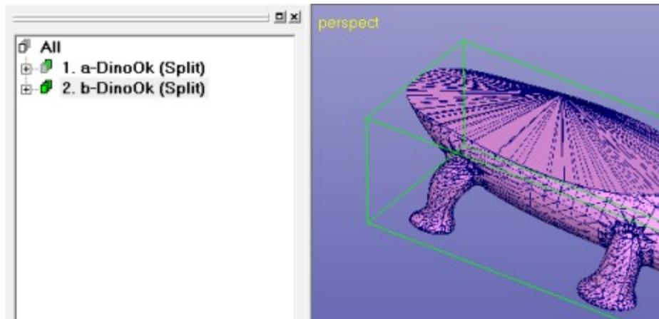
The pins are now **created with the *Print Preparation > Connect* command** or using the Print Preparation Tab shortcut
