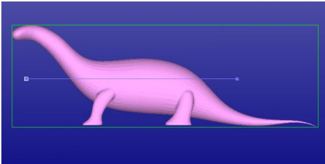
The curve editing is finished by **pressing the RMB** (or *ESC* key to cancel). When RMB is pressed the model is split along the plane defined with the polyline. After a while the result is available in the Model Tree. You can select the upper part with LMB click on the shell *1. a-dino (Split)* to highlight it.
