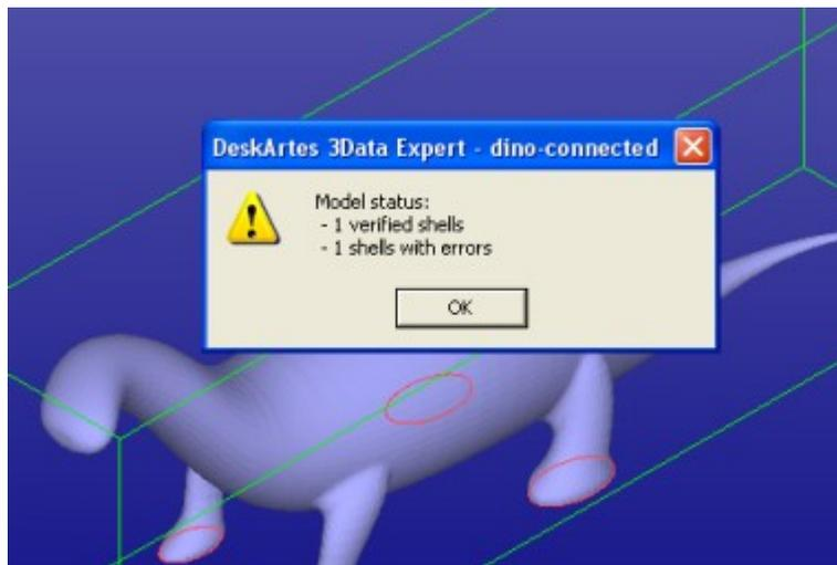
The message indicates that there is one verified shell, which also contains errors. The display shows red *Gap curves* through the surfaces. Gaps are an error type you must fix during the repair process.
