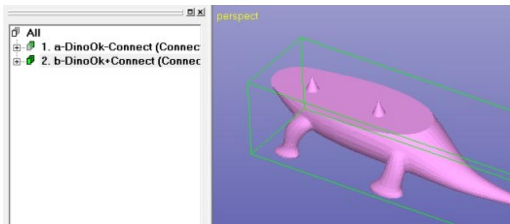
Corresponding holes are automatically created to the *a-DinoOk-connector* shell.
