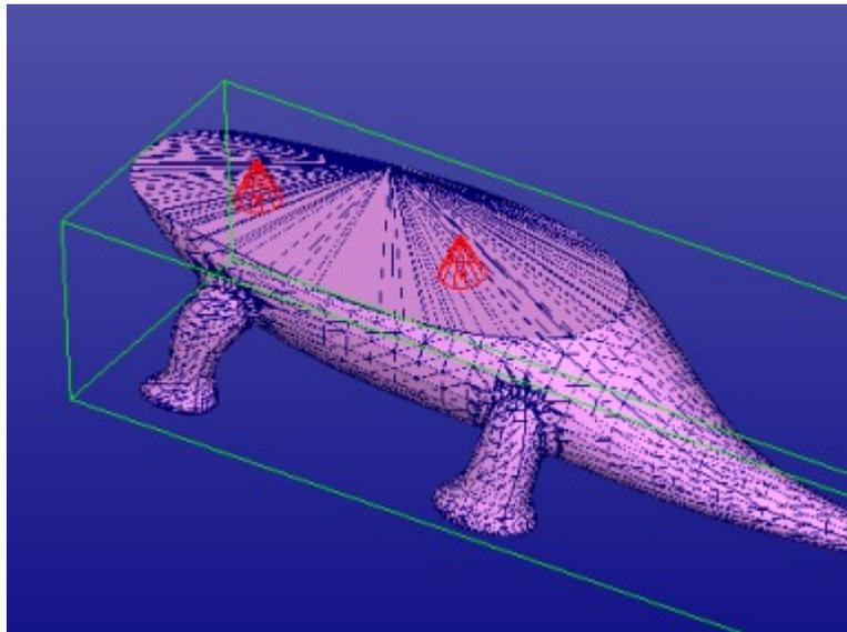
When ready **Press OK to generate the connectors**. After a while you will see the connectors added to the selected shell (in shaded mode again with
