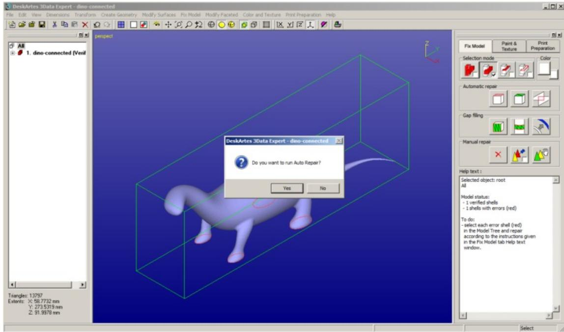
Auto Repair is the best path to follow when repairing everyday models. Auto Repair will attempt to fix all shells with errors in the Model Tree. Especially when you only have one shell, like now, you should always try Auto Repair first. **Press the Yes button** to initiate Auto Repair now.
