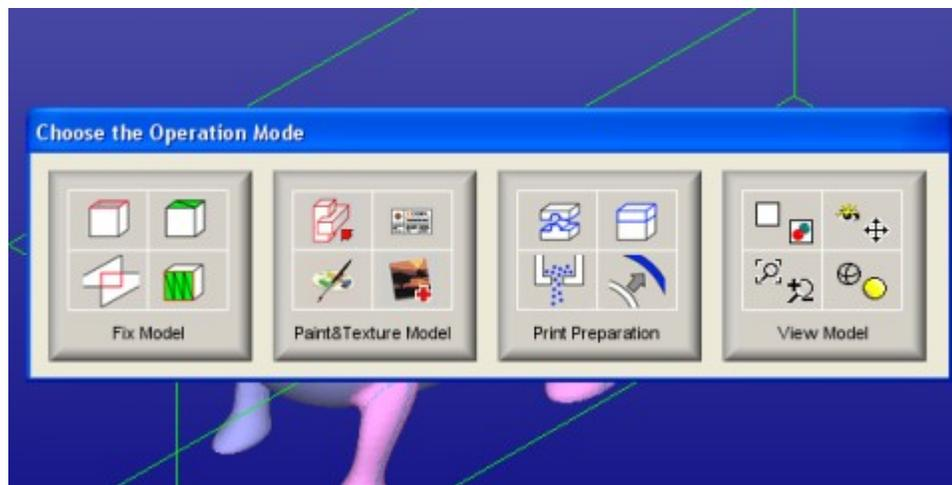
The normal way to begin repairing a model is to start with the Fix Model mode. To start fixing **press the Fix Model button** in the Operation Mode dialog now. *Expert Series* will begin automatic model verification (*Fix Model > Verify Shells* command). The screen is erased and a progress bar appears. When the analysis is ready, a *Model status* message box is displayed
