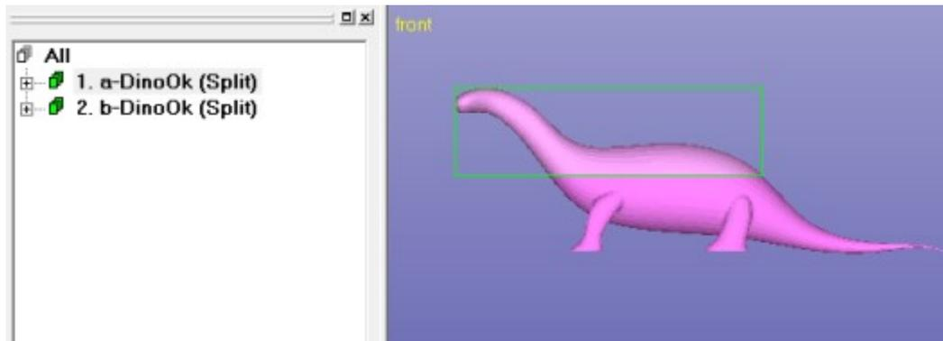
The two halves are named with *a-* and *b-* prefixes to distinguish between the shells above the split line and below the split line.
