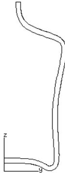
The curves are joined to form one single curve which defines both the outside and inside of the bottle.
