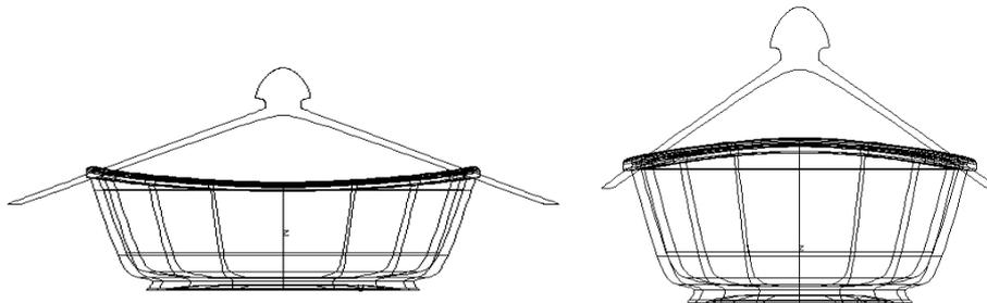
Finally create a cutter as an extrusion of an Xprojection and chop of the excess of the lid.
