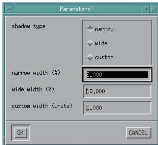
The size of the light source can be selected as **Narrow**, **Wide** or **Custom**. With wide and narrow you can set the size as the percentage of the whole model size ("universe"). The custom size is specified directly in the same units you are working in with the model.
