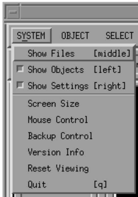
To **select a command** from a pull-down menu, point the cursor at the desired menu title and hold down the left mouse button. Still holding the button down, drag the cursor to the desired command. **Execute** the command by releasing the mouse button.
