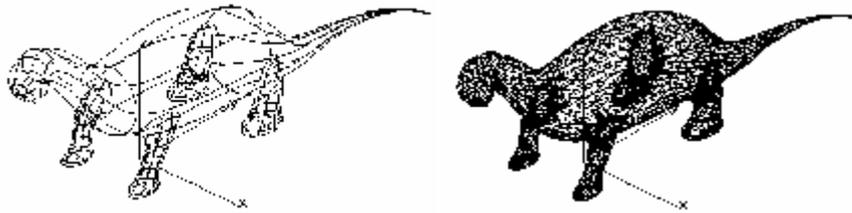
A parameter box appears requesting a *tolerance* for the faceting. This determines the *maximum distance* of the facets from the actual surface(s).
