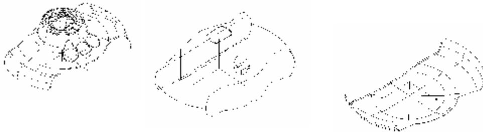
If there exist vertical walls within the model, the user must decide if they represent design errors or if they can be used for the mold. In the latter case, the user can interactively place them from the “parting” element into the “upper” or “lower” elements using OBJECT⇒ Cut & Paste.
