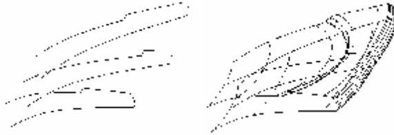
This portion of the plate rim was then copied and rotated by 30 degrees around Z 11 times to form the complete rim.
