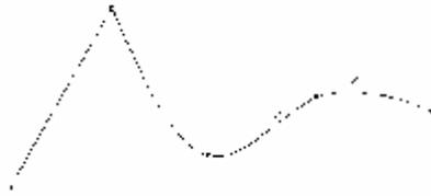
With the command `CURVE⇒Design: Edit` you may move the Bézier control points and handles, add new control points without changing the shape of the curve, define arcs and fillets, and further manipulate the curve shape.
