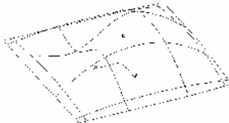
The B-spline surface is able to assume a variety of shapes that do not appear to resemble the rectangular patch structure at all. For instance, a sphere may be made and the 'rectangular' patches become like lines of longitude and latitude.
